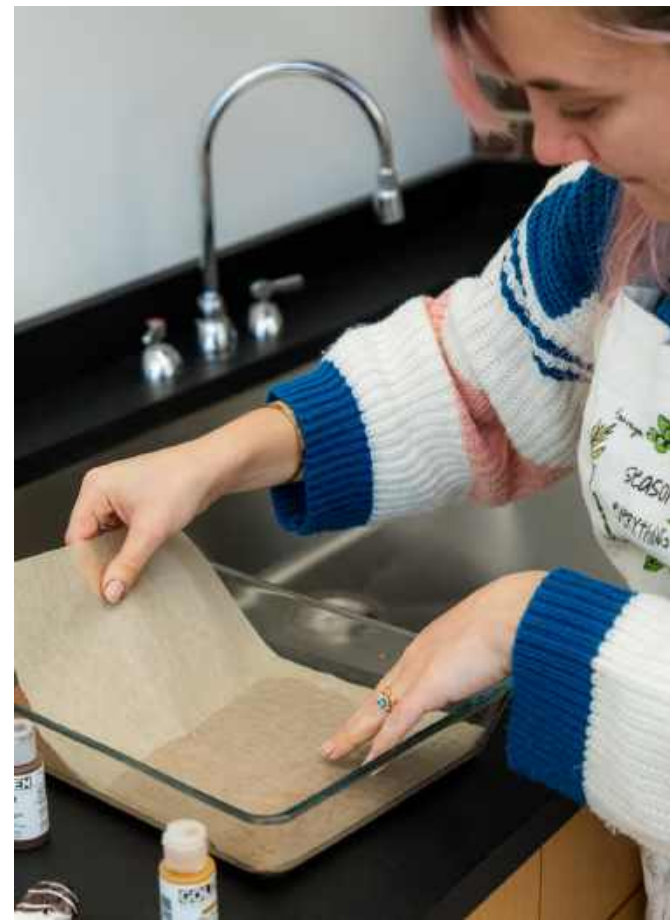
Library and Archives Conservator Marissa Maynard dyes mending tissue for paper repair in the Conservation Lab.
