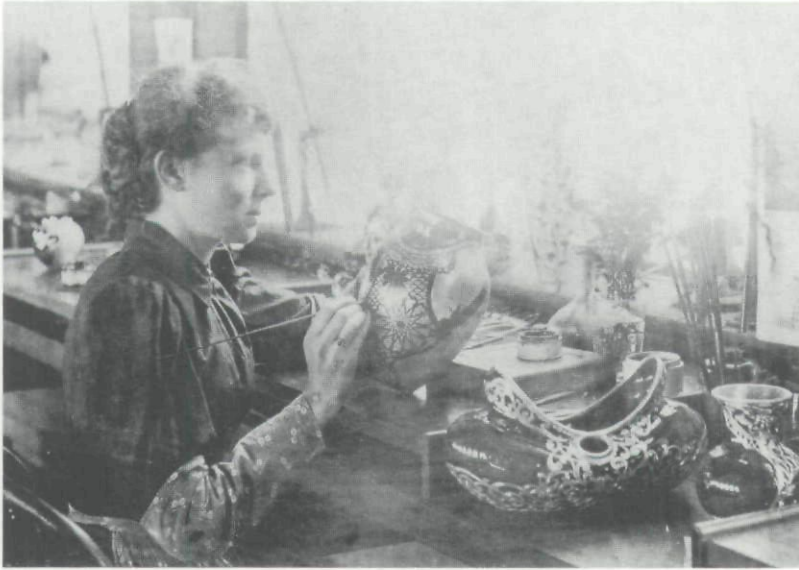
Fig. 1. A Gorham artisan etching silver, c. 1892. The worker shown here is carefully painting a nonconductive resist varnish over a perviously drawn pattern or scene. After this, the piece would be dipped into an acid bath to corrode away the unvarnished surface leaving the varnished design in relief. The protective varnish would then be removed, and the pattern would stand out in relief. This process might be repeated three to four times to achieve a pattern of varying depth. Women with drawing and painting skills were considered most likely to succeed at this task. Women's Work at the Gorham Manufacturing Company , 1892. Brown University Library.
