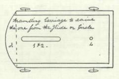
A bolt threw the upper carriage to play into & 2, to slide out longer for a stern chase, if necessary, & the sweep of 3, may lodge on the stern sill, prevents its tipping up & when for a side gun a bolt in 4 will steady it firmly.
